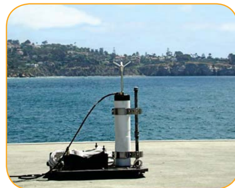
A Triton-ADV ready for deployment off La Jolla, California.
