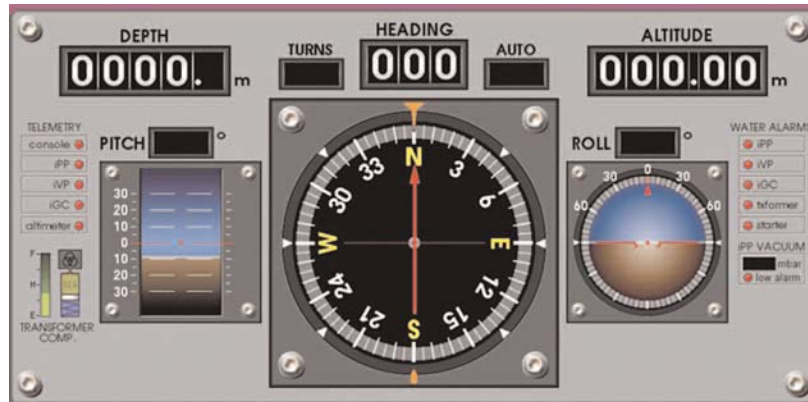
Custom iVP (Intelligent Valve Pack) display, showing iGC heading, pitch and roll.
