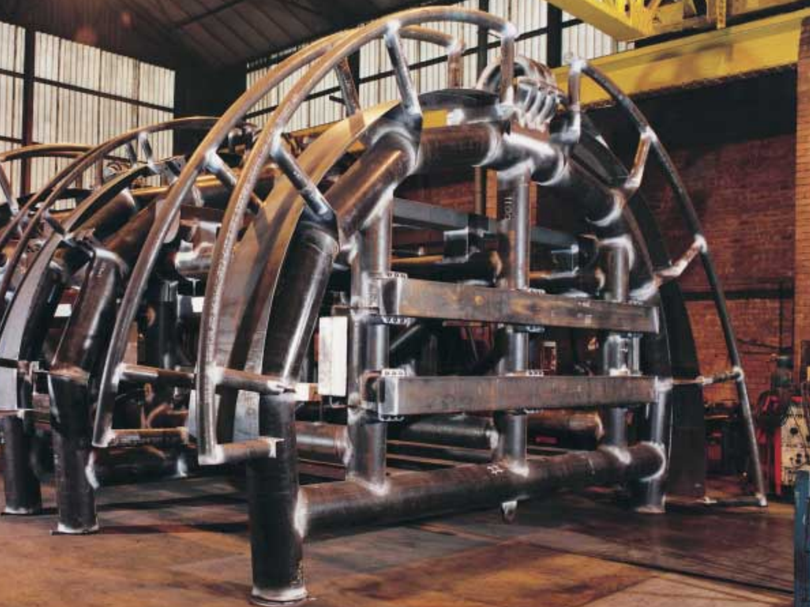
Complete Arch 'skeleton' ready for first stage of the coating process
