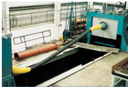
Trelleborg CRP Bending Stiffeners undergoing dynamic testing
