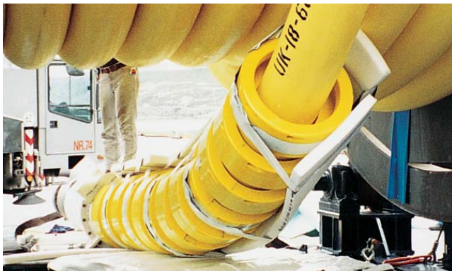
Pre-installed Bending Restrictor on flexible pipe reel
