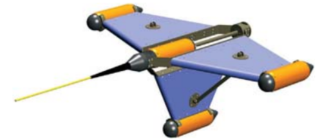
3-sensor biaxial gradiometer for very shallow water
