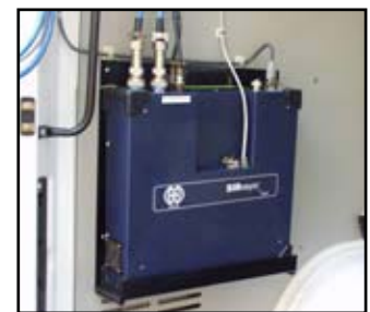
SIR-20 shown with computer mounted in the front of vehicle and GPR control unit mounted in the back.
