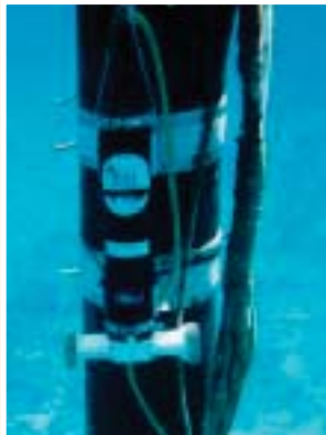
▶ NXIC-CTD Bio-Auto-500M installed on NOAA's Coral Reef Early Warning System (CREWS), Lee Stocking Island, Bahamas.
