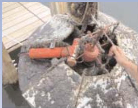
▶ NXIC CT Sensor interfaced to an FSI 2D ACM in a TRBM deployed in Packery Channel near Corpus Christi Bay, TX. Photo courtesy of the Shoreline Environmental Research Facility of Texas A&M University. www.serf.tamug.edu
