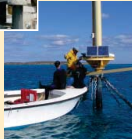
▶ NXIC-CTD Bio Auto-500M installed on NOAA's CREWS buoy, Lee Stocking Island, Bahamas.
