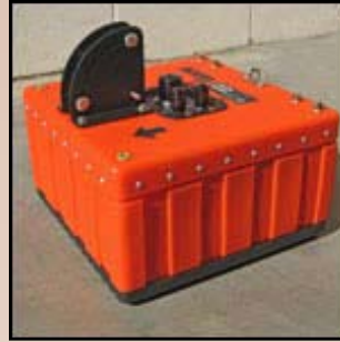
0 - 12 feet 400 MHz Antenna
