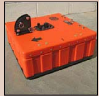
0 - 18 feet 270 MHz Antenna
