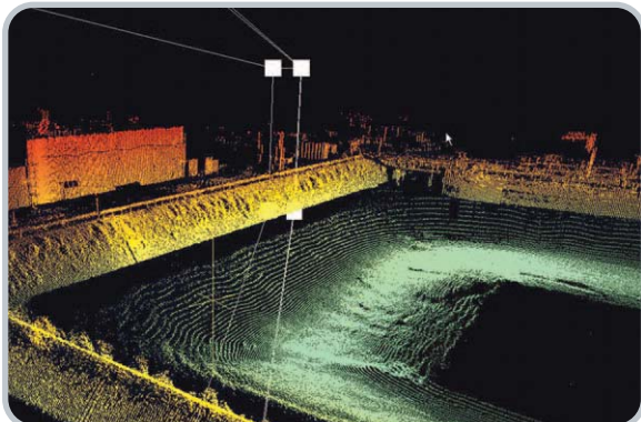
Combined laser and bathymetric data from a harbour survey
