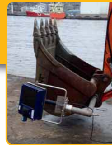
Echoscope mounted and deployed with excavator bucket
