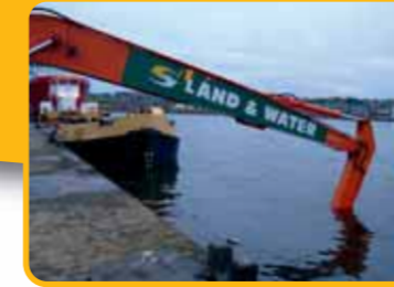
Echoscope mounted and deployed with excavator bucket
